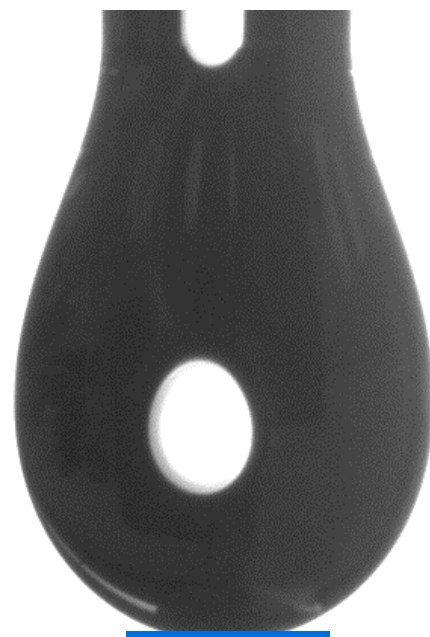
Pendant Drop for Interfacial Tension
