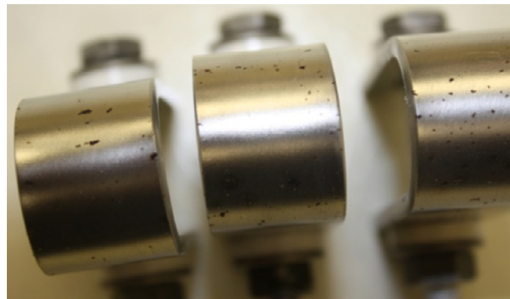
CNWRA measured corrosion rates of stainless steel used for spent fuel storage canisters to evaluate the potential effects of airborne salts.
