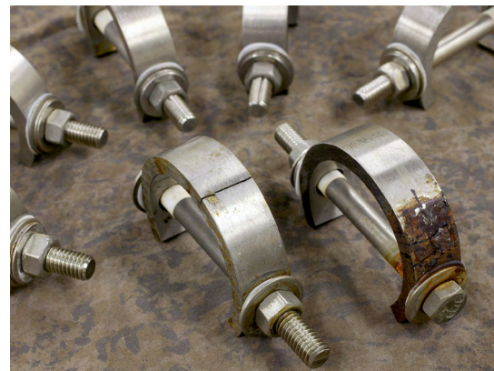
SwRI performed stress corrosion cracking (SCC) evaluations using C-rings. Specimens were exposed to a downhole simulated environment and evaluated for SCC.
