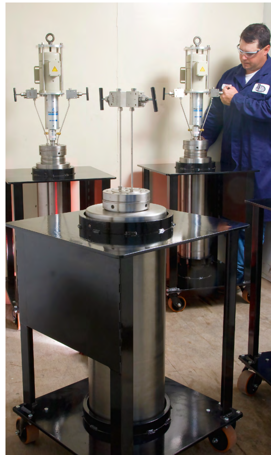
High pressure high temperature (HPHT) testing can be performed to determine stress cracking and/or mass loss corrosion effects under H_2S , CO_2 , or other gaseous environments. Testing can be performed up to 650°F and 20,000 psi.
