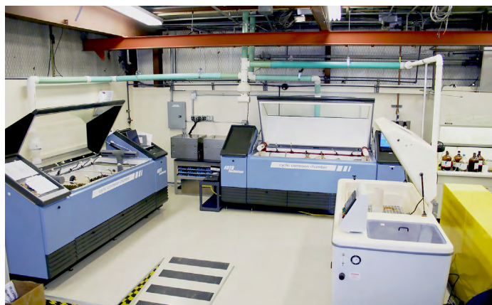
Precipitation and particulate chemistry, wet and dry deposition, and cyclic corrosion are some of the important factors measurable using the EPM Lab's three environmental corrosion chambers.
