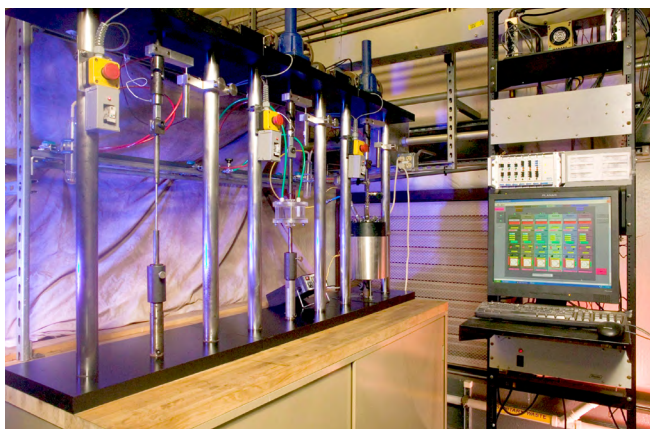
Slow strain rate (SSR) testing is used to determine cracking susceptibility in various environments including high pressure and high temperature.
