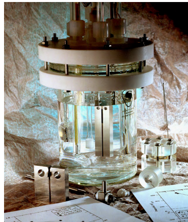
Testing and evaluation of corrosion rate, galvanic corrosion, uniform corrosion, impedance and pitting corrosion are a few examples of the extensive electrochemical testing capabilities testing program at SwRI.
