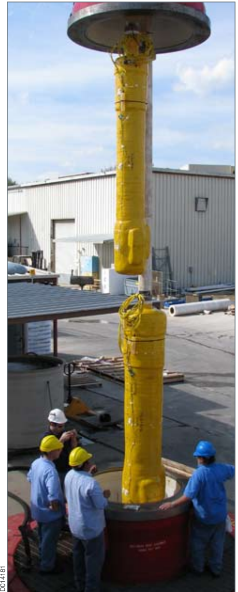
Simulated service insulation test samples being set up for pressure/temperature test
