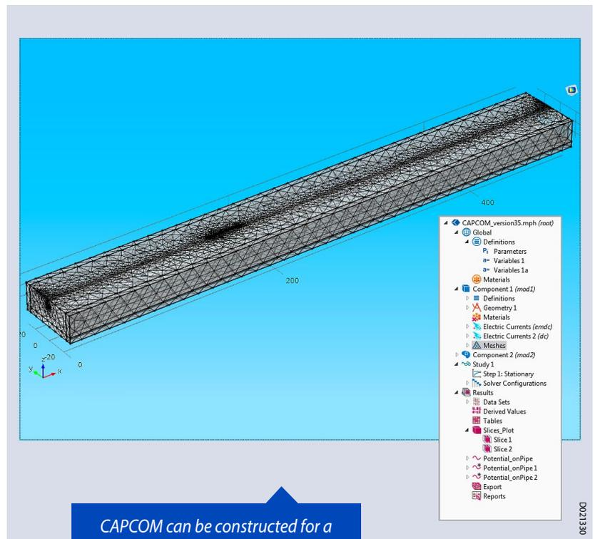
*CAPCOM can be constructed for a specific set of geometric parameters and field conditions. The constructed model can be visualized using the graphical user interface.*
