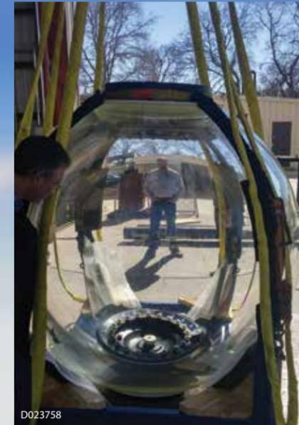
SwRI pressure tested this commercial submarine acrylic sphere in our **90-inch, 18-foot-deep** pressure chamber to ensure that it would withstand sea pressures without leaking.
