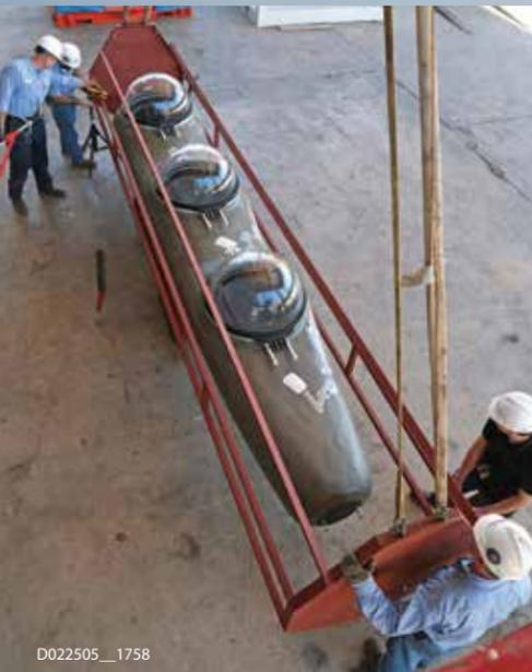
Engineers used an array of strain gauges to evaluate the pressure hull and dome windows of this deep-sea **3-man** submersible tested in SwRI's high-pressure chamber.
