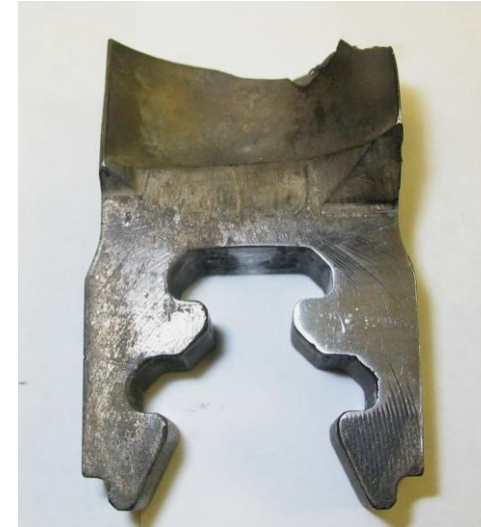
Blade failure from high cycle fatigue cracking
