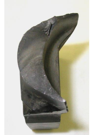
Blade failure from high cycle fatigue cracking
