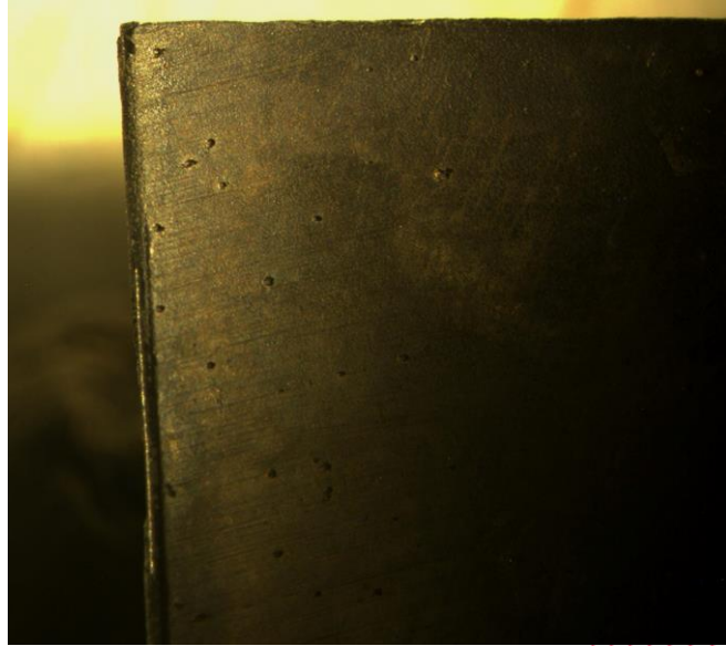
Corrosion Pitting on surface of geothermal steam turbine blade
