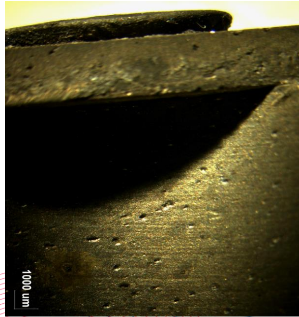
Corrosion Pitting on surface of geothermal steam turbine blade
