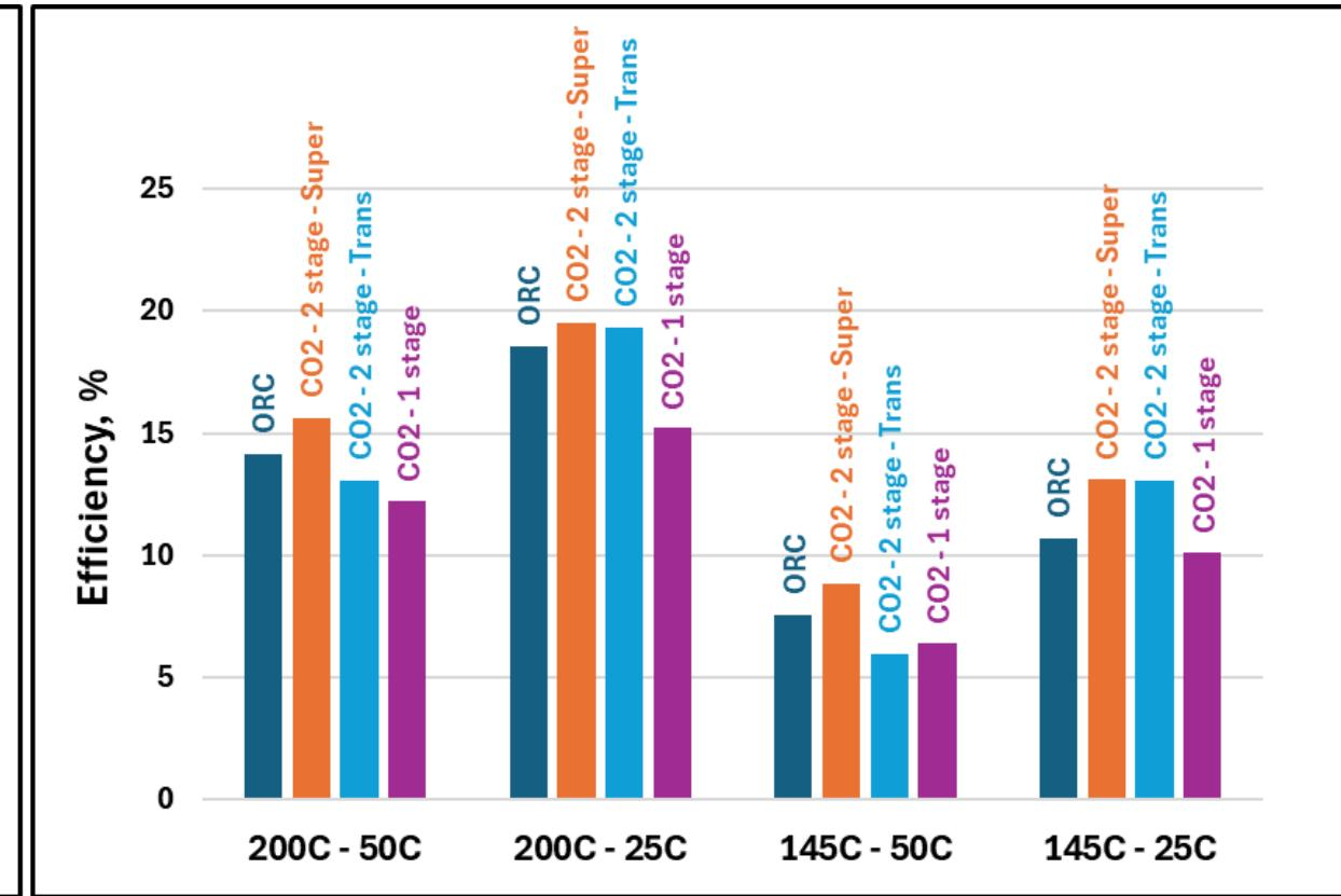
*sCO<sub>2</sub> Brayton cycle provides maximum net power output for the entire geothermal temperature application range*
