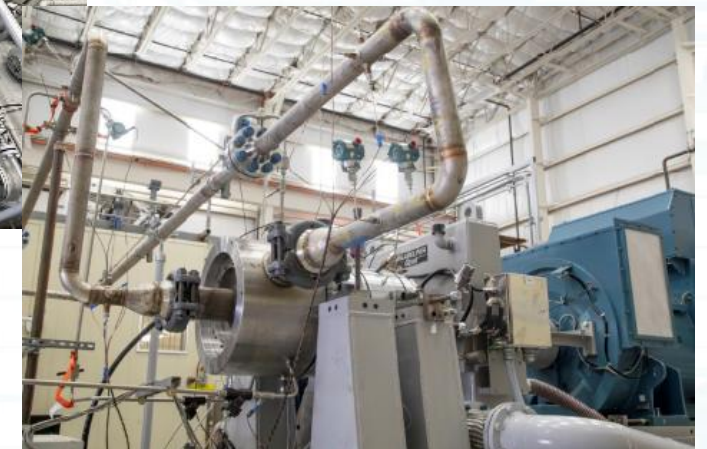
Sage turbine on test stand
