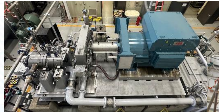
Sage turbine on test stand
