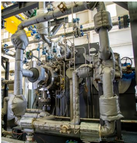
Hanwha Integrally-Geared 10 MWe-scale Radial Turbine/Compressor: Test at 720 °C, full-flow compressor 1/10 flow turbine
