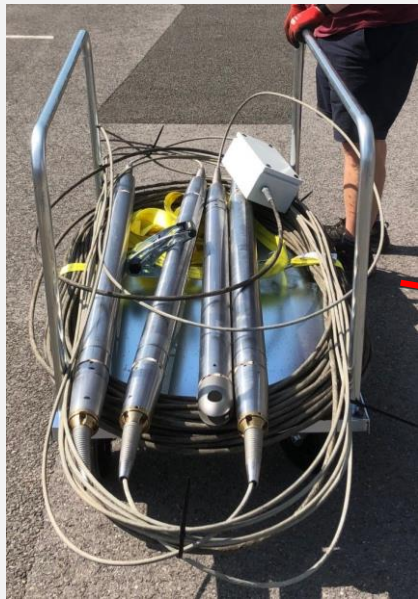
3-level, 3C fiber optic string with wireline DAS
