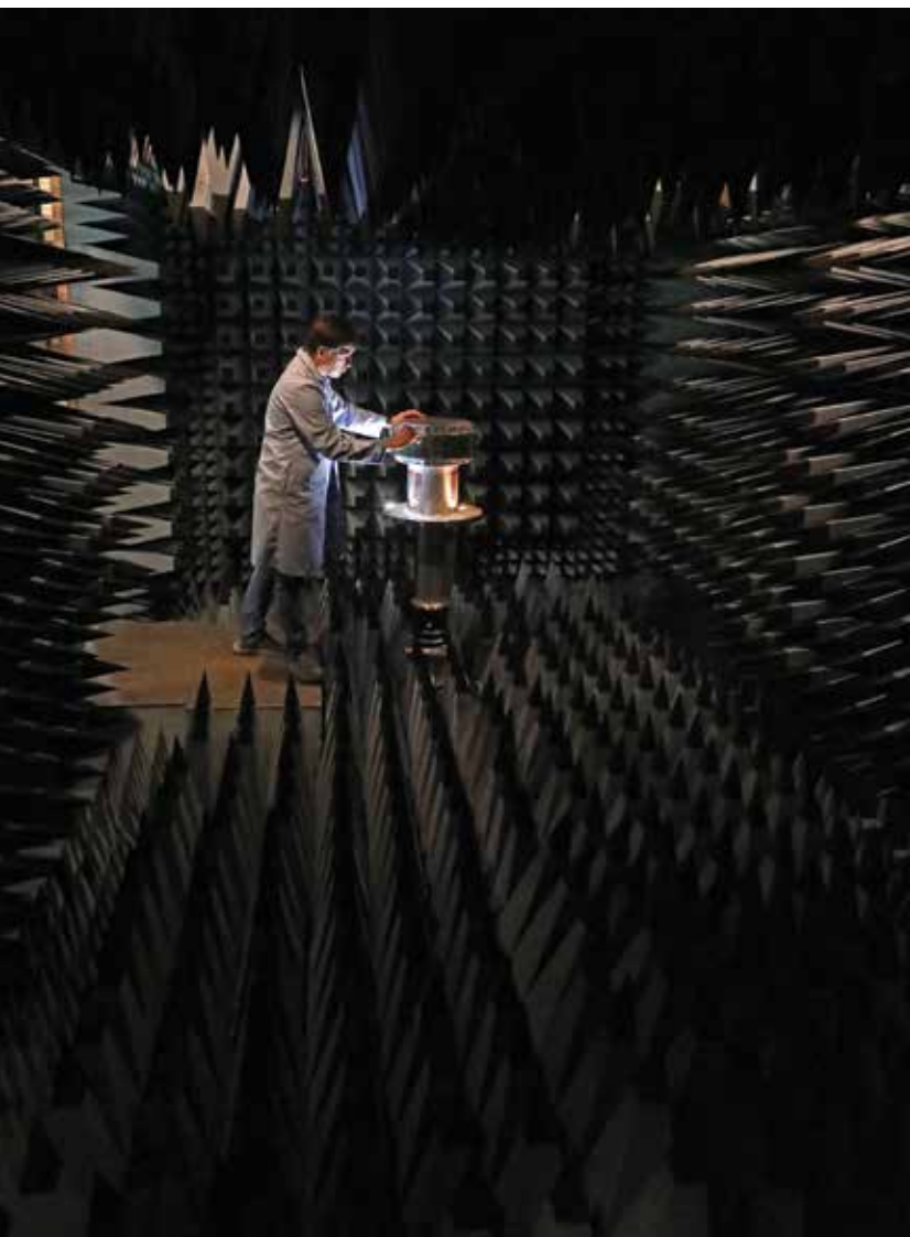
In 2020, engineers evaluated new antenna technology in our anechoic chamber. The SwRI-designed cylindrical slot array demonstrated high-quality omnidirectional output while also performing well as a DF array.
