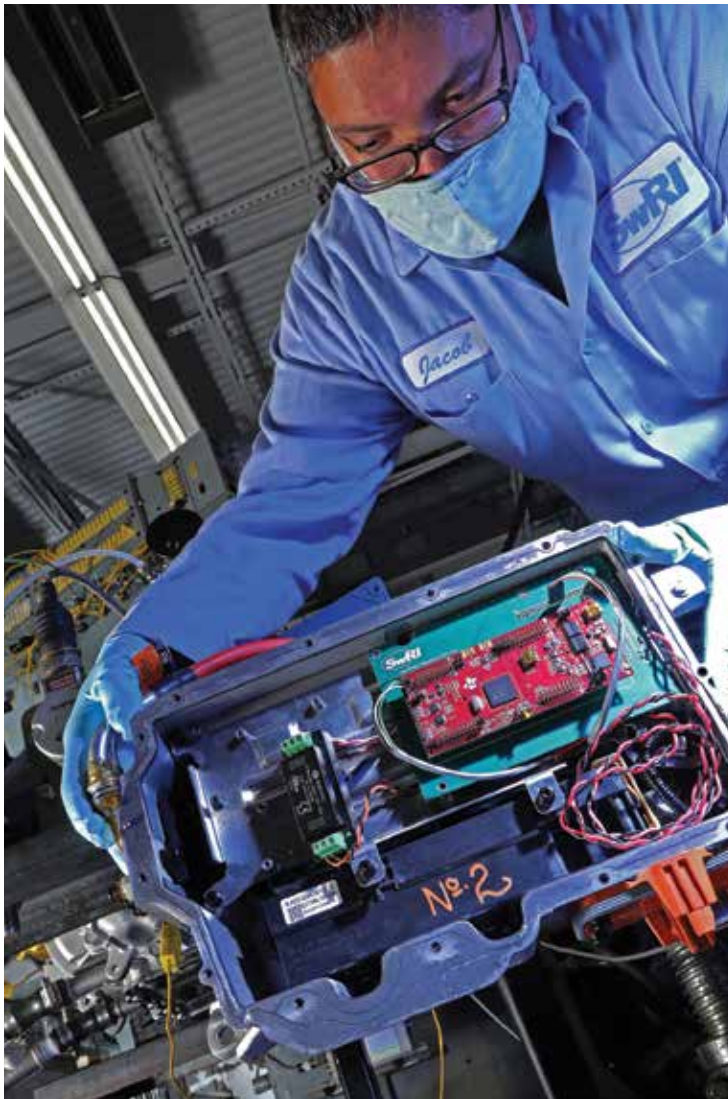
SwRI developed this sophisticated open inverter, which runs any electric motor to OEM specifications without OEM support and can evaluate client parts or fluids for electrified powertrains on various hardware.
