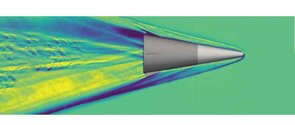
Using SwRl's two-stage light-gas gun to simulate hypersonic flight, engineers study the shock wave velocities around the flight body, using techniques including the false-color schlieren image shown here.
