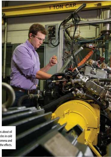
As hybrid vehicles proliferate, SwRI is addressing concerns about oil emulsions forming in association with short drive cycles in cold weather, developing engine tests to replicate these phenomena and evaluate whether different formulations could mitigate the effects.
