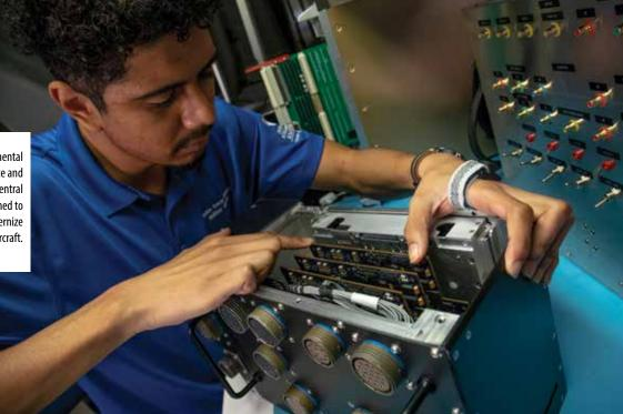
In 2021, SwRI conducted environmental and electromagnetic interference and compatibility testing of A-10 central interface control units, designed to replace legacy systems and modernize aging aircraft.
