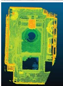
At an industry challenge event, SwRI demonstrated autonomy technology for an unmanned aircraft system, successfully navigating a nonoperational nuclear facility to locate radiation sources hidden inside. SwRI's drone-based system uses novel algorithms and computer vision to autonomously explore and map unfamiliar environments.
