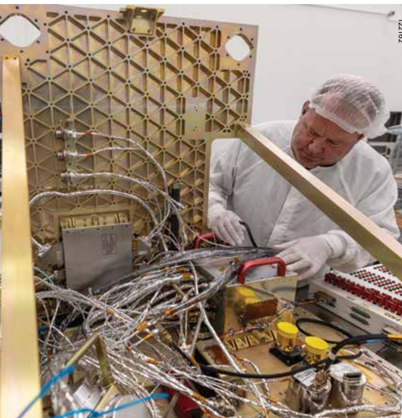
▼ SwRI is building QuickSounder, the first of a new generation of NOAA low-Earth orbit environmental satellites, which will deliver 95% of collected data within 30 minutes to significantly improve weather forecasting.
