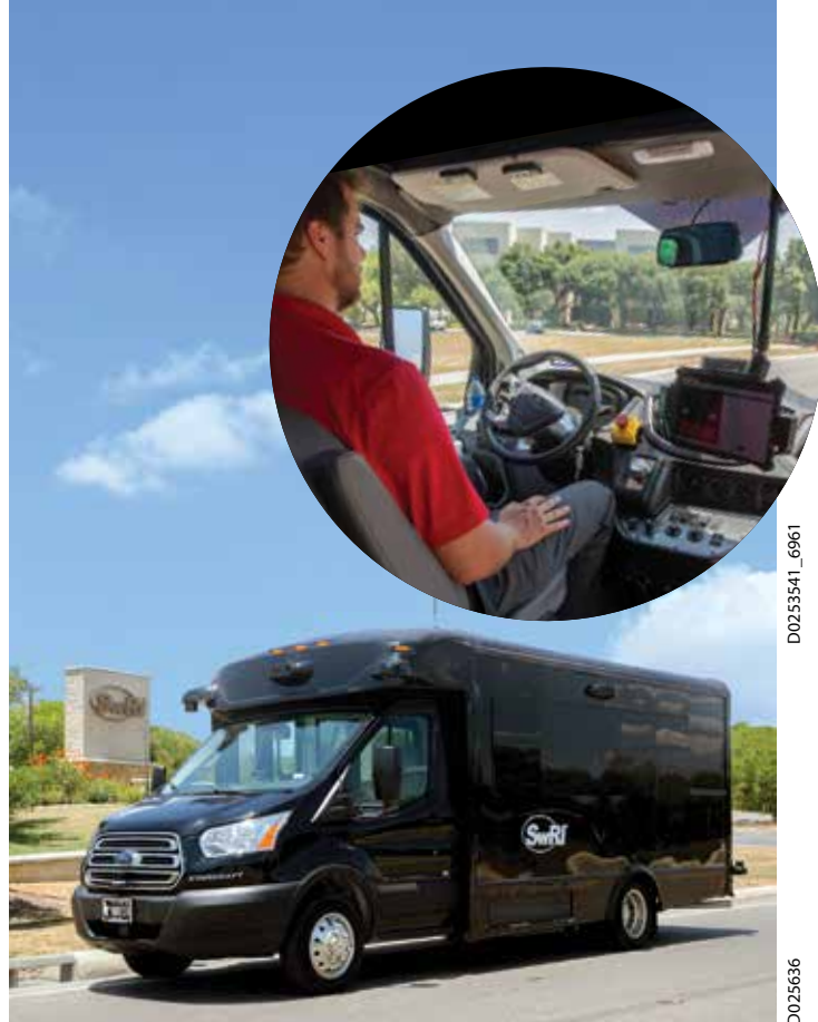
A key component of an ADS is the visualization technology that allows a vehicle to navigate while recognizing objects, traffic signs, pedestrians and other vehicles. The team continues to enhance and improve the capabilities of these systems using platforms such as an automated driving shuttle that runs regular routes around SwRI's 1,500-acre San Antonio campus.
