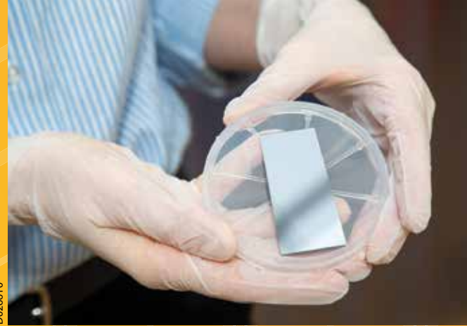
SwRI space scientists collaborated with materials specialists to create more effective particle detection surfaces for spacecraft instruments. Pictured is a conversion surface substrate developed specifically for the IMAP-Lo instrument.
