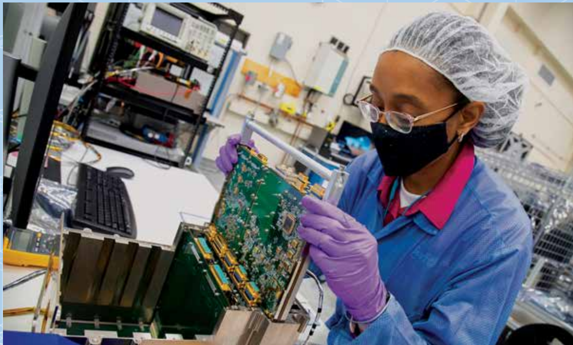
Engineers integrate the electronics box for SwRI's novel MASPEX instrument, which will sample gases in Europa's faint atmosphere and possible plumes of materials escaping from surface cracks to determine the chemistry of the moon's surface and internal ocean.
