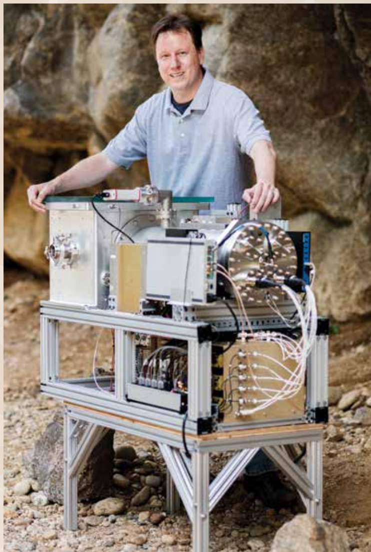
Institute Scientist Dr. Scott Anderson stands behind the SwRI-developed laboratory prototype mass spectrometer for the CODEX instrument, which allowed the team, with IR&D support, to determine the optimal operational parameters for the instrument. The instrument has since been demonstrated with an even smaller miniature mass spectrometer from the University of Bern.
