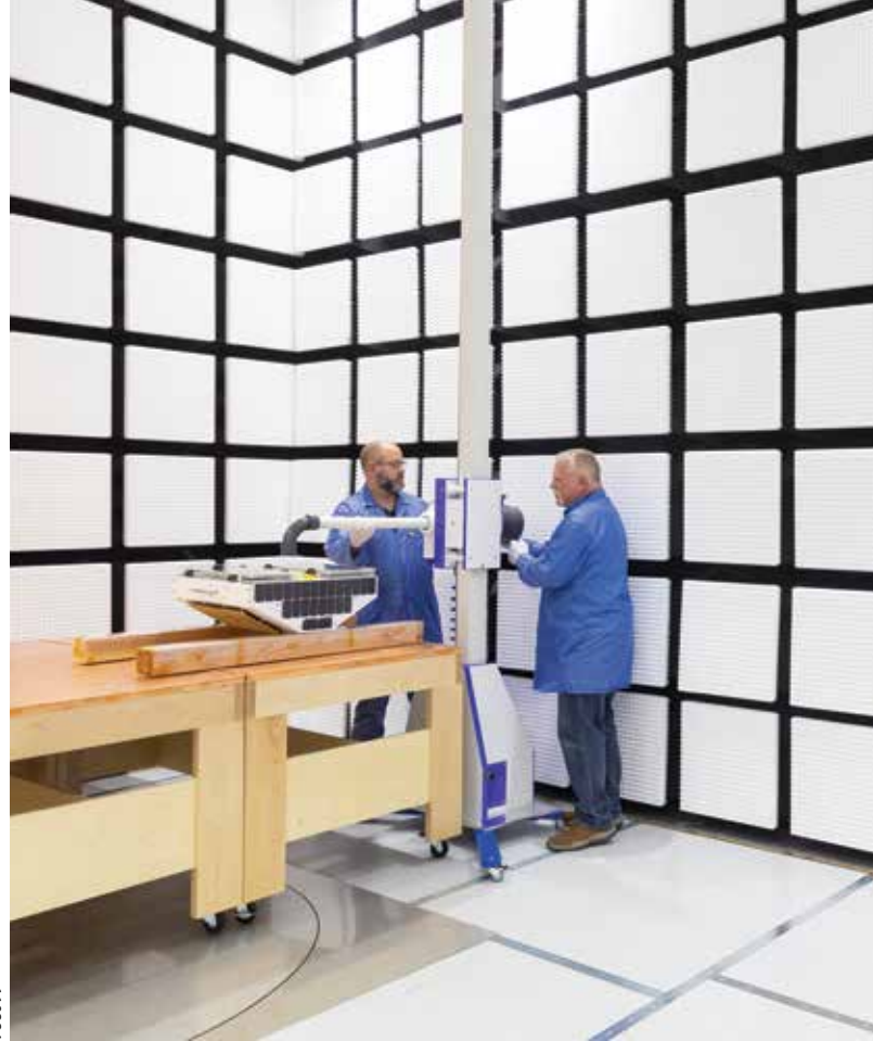
SwRI’s new semi-anechoic shield enclosure is designed to perform EMC/EMI and radio frequency testing for spacecraft.
