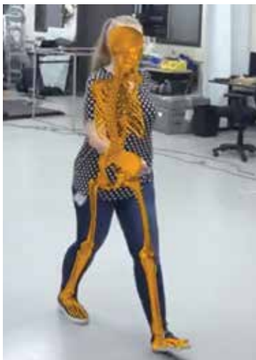
Using the ENABLE markerless biomechanics system, SwRI can accurately and automatically quantify a person's detailed 3D movement from video. This comprehensive full-body gait analysis can capture kinematic variables in the hips, knees, ankles, shoulders, elbows, etc.
