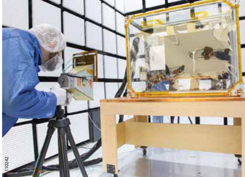
SwRI evaluated the PUNCH spacecraft in a new electromagnetic compatibility and interference test chamber. This vital testing happens just feet from the fabrication area, saving costs, increasing efficiency and decreasing risk of damage in transit.
