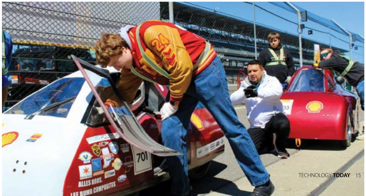
SwRI's Jose Starling (in white) checks the urban concept BEV designed and built by Team RUDI from Mater Dei High School. Team RUDI placed first in their category reaching an efficiency of 120.38 mi/kWh.
