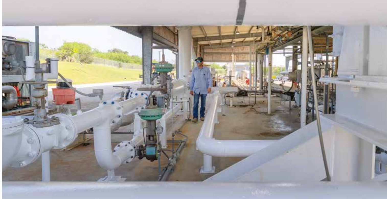
SwRI upgraded its Metering Research Facility to help several industries evaluate how blending hydrogen with natural gas affects infrastructure and technology.
