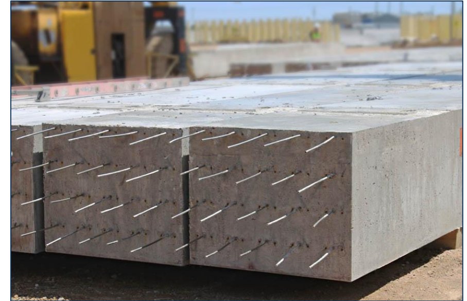
Storworks concrete BolderBlocs with embedded steam tubing
