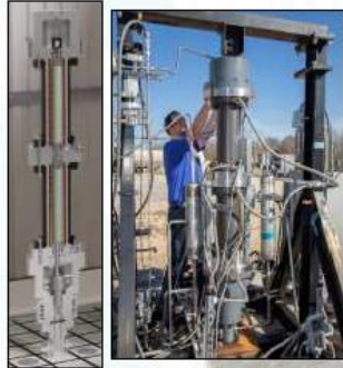
Hydrogen Compressor Development and Test Loop
