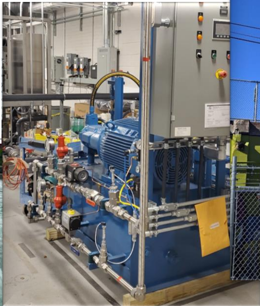
CO 2 heat pump & power cycle
