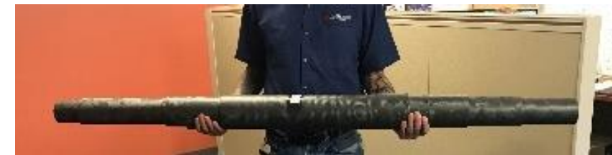
Continuously wound carbon fiber in epoxy matrix through additive process
