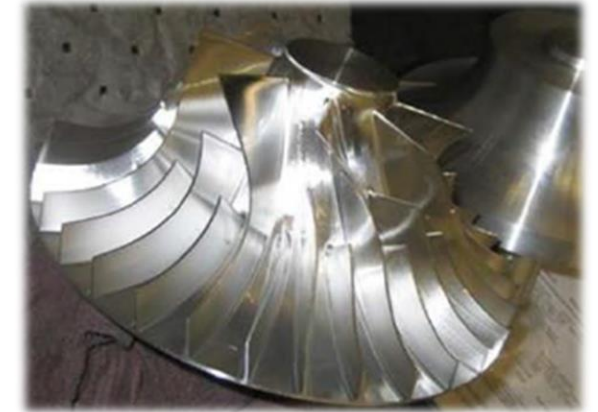
NREC 2,100 fps 7075-T6 Aluminum impeller
