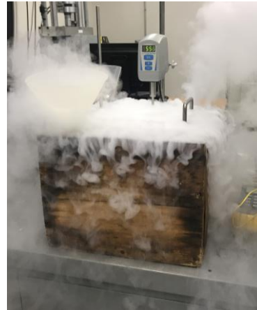
Charpy V-Notch Impact Specimen submerged in cooling bath at required testing temperature
