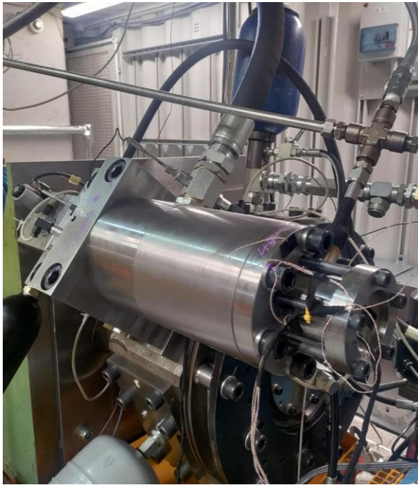
Prototype test rig ~60kWe Running for ~1 year
