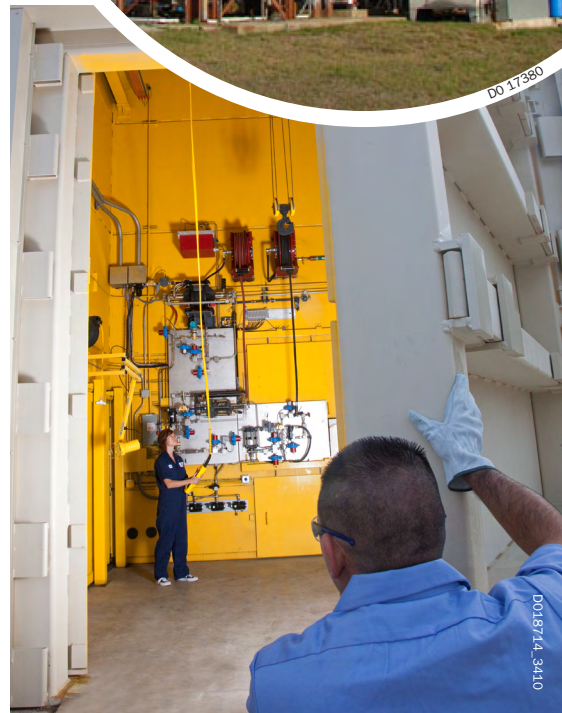
All high-pressure tests are conducted within large containment chambers to allow for safe operation.
