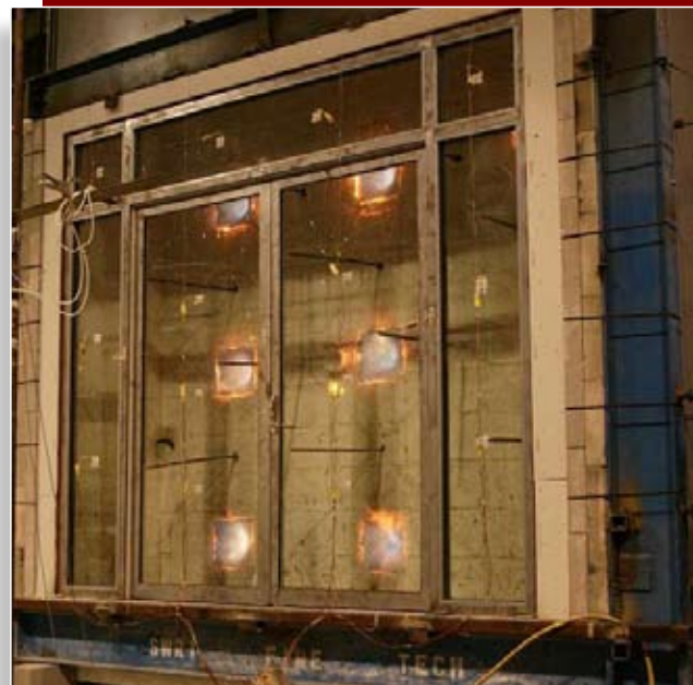
Glass wall and double door assembly being tested on SwRI's large-vertical furnace
