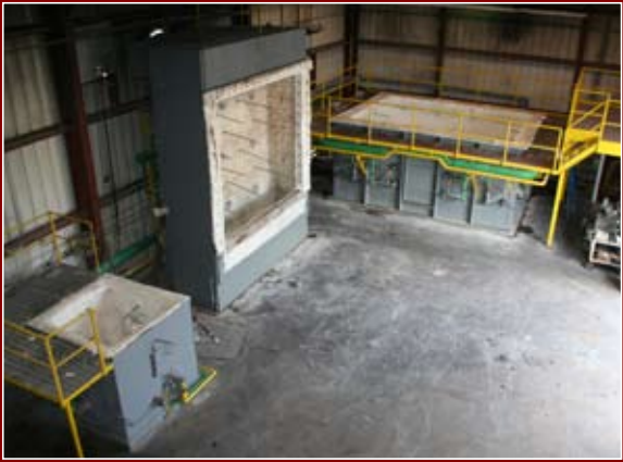
SwRI's three furnaces (left to right): small-horizontal, large-vertical, and large-horizontal
