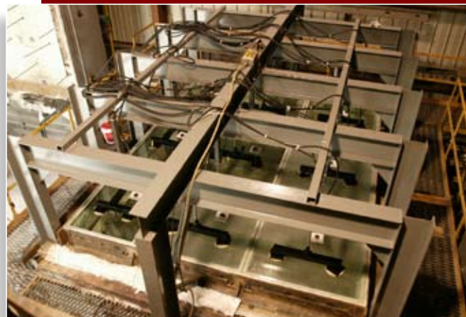
SwRI's loading frame for the large-horizontal furnace applied over a glass floor system
