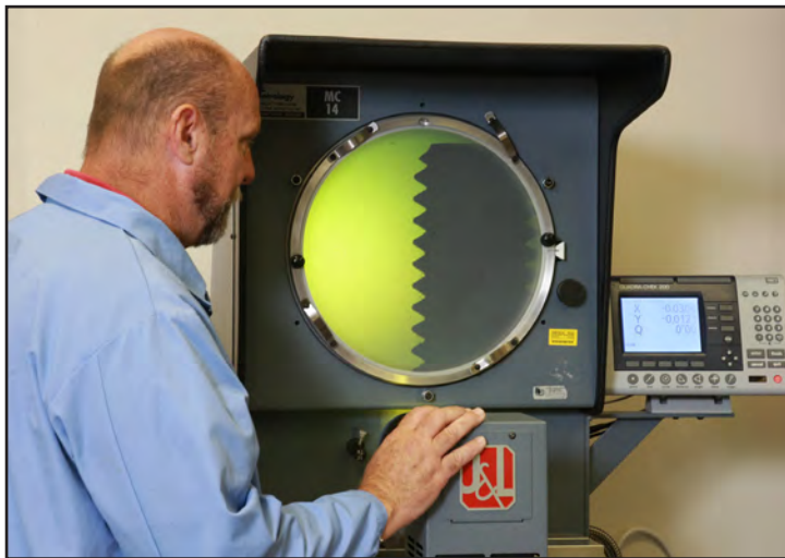
J&L 14" Optical Comparator. This machine produces a magnified silhouette of a part using either a 10-, 20-, or 50-power lens plus surface reflection. The silhouette is projected onto a screen and from this silhouette, measurements of the geometric shape of the part and its dimensions are collected.
