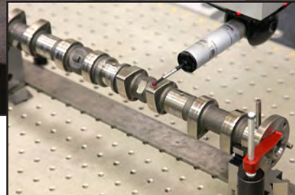
Brown & Sharpe® Global Image Coordinate Measuring Machine (CMM). The CMM measures the physical geometric characteristics of an object using its x-, y-, and z-coordinates to determine its size and position. This machine may be manually controlled or controlled by a computer. This machine also allows technicians to import computer-aided design (CAD) models and measure a component from the model.
