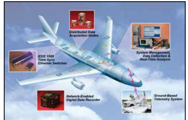
SwRI has developed solutions for aircraft-wide distributed flight test data acquisition systems.
