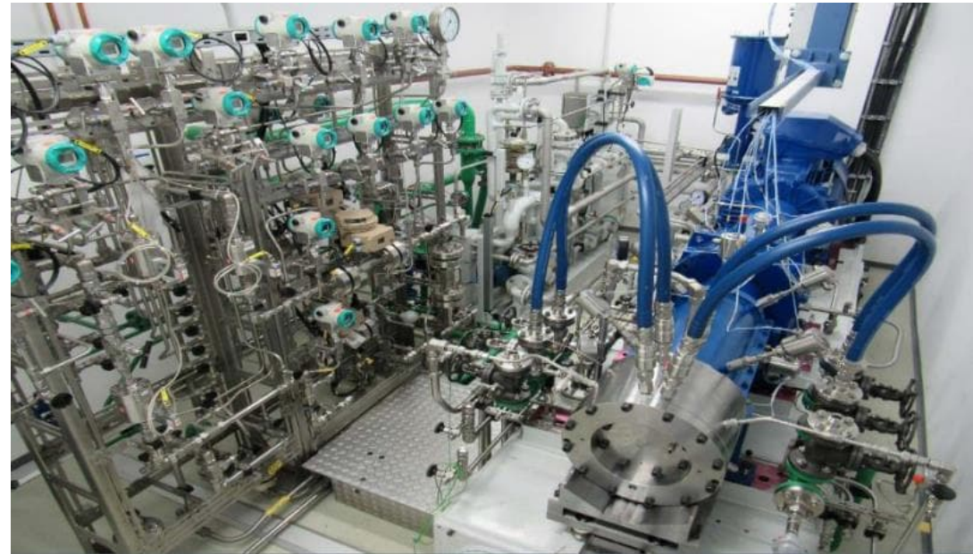
Siemens Energy DGS on Test Stand
