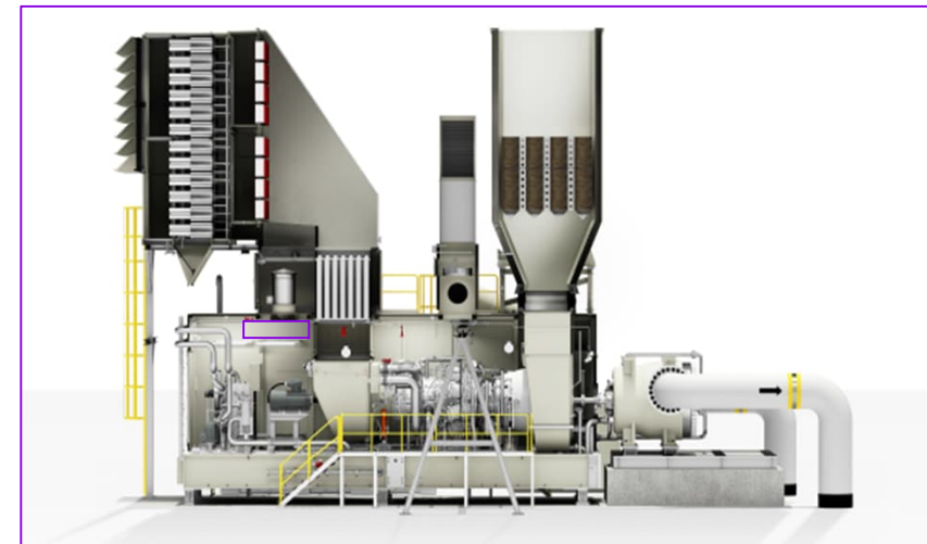
Typical Gas Turbine driven Compressor (GTC) Train
