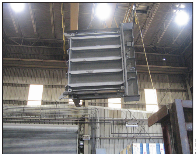
SwRI designed and built a custom pressure containment chamber to pressure test both sides of a water-tight door for a semi-submersible production platform.
