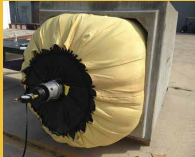
The POD field-deployable system includes this inflatable structure designed to thwart the passage of individuals or vehicles by blocking large openings or tunnels.
