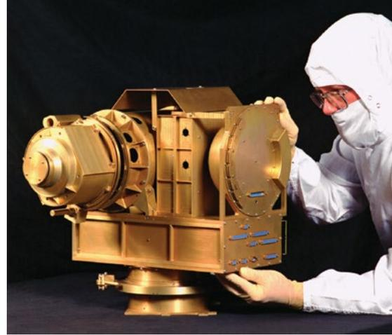
SwRI operated two of Cassini's 12 science instruments, as part of the fields, particles, and waves experiment package. The Cassini Plasma Spectrometer (CAPS), above, and the Ion and Neutral Mass Spectrometer (INMS), below, both studied plasma in the Saturn system. While they didn't produce actual "pictures," the information they collected is critical to scientists' understanding of the Saturn system, including its moons and rings.
