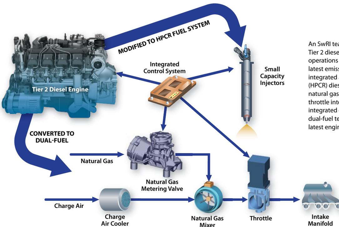
An SwRI team explored modifying a Tier 2 diesel engine for dual-fuel operations to cost-effectively meet the latest emissions standards. The team integrated a high pressure common rail (HPCR) diesel fuel injection system and natural gas control valves, mixers, and throttle into the non-road HD engine. An integrated control system tunes the new dual-fuel technology to meet the EPA's latest engine emissions standards.
