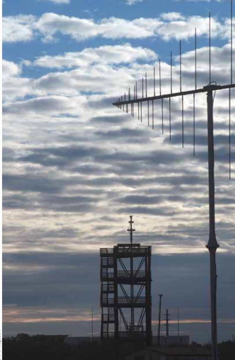
SwRI's 200-acre antenna test range includes two 70-foot towers to simulate and evaluate antenna systems on the masts of naval vessels at sea.
