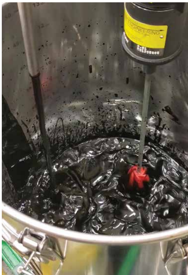
To demonstrate the EZ Flow process at a bench scale, chemists heated a heavy crude sample to 40°C in a stirred-stainless-steel, conical-bottom vessel while sequentially mixing low-concentration chemicals into the heavy crude oil.
