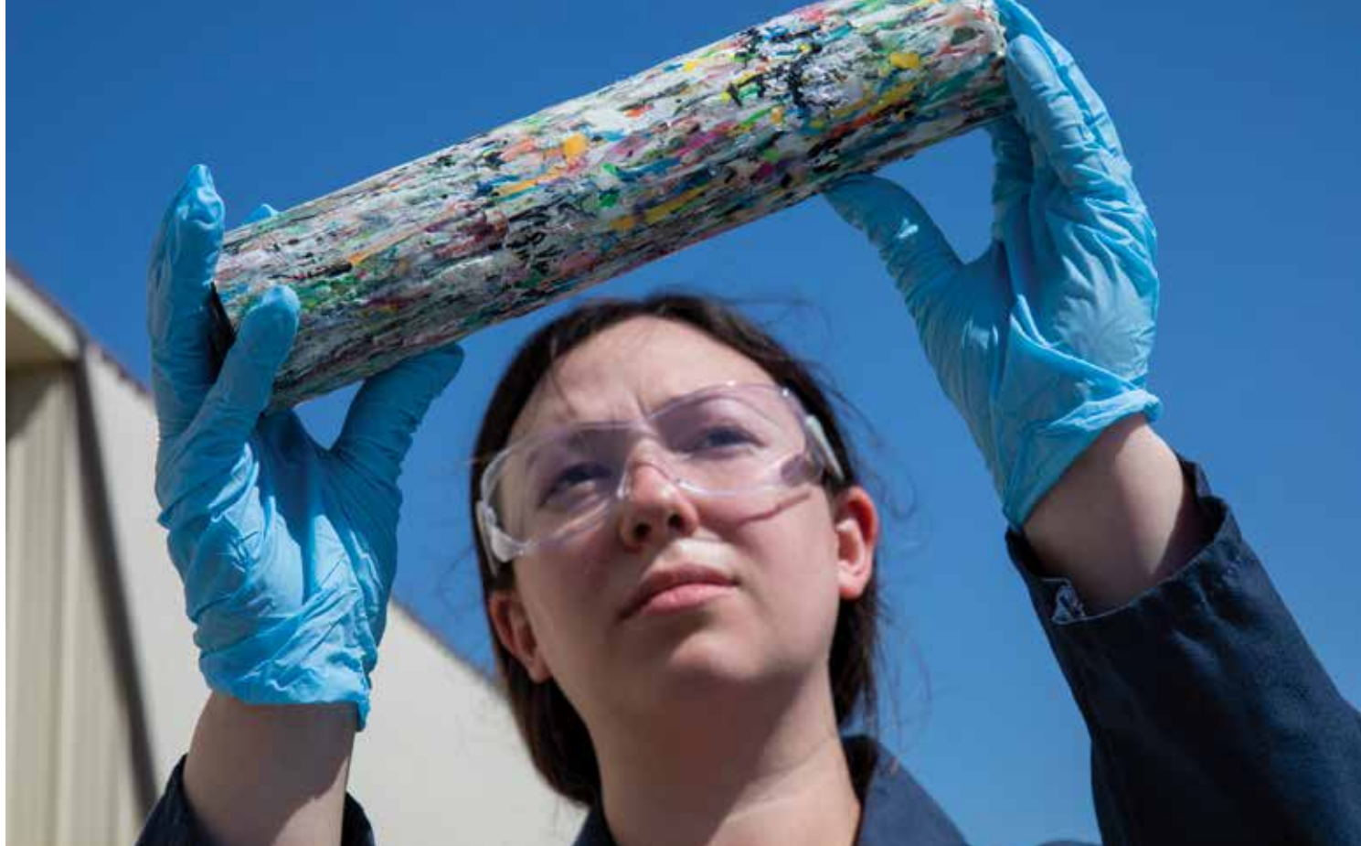
New SwRI-developed processes are chemically recycling mixed plastics, shown melted together into a cylinder, to target the large number of plastics in our economy that are currently not being recycled.
