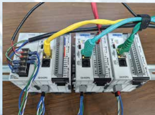
Using a bench test network, SwRI-developed algorithms scanned data packets transferred via the Modbus/TCP protocol for cyberattacks.
