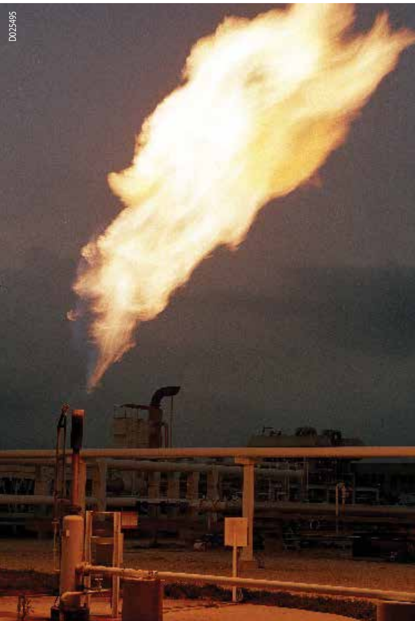
SwRI's MRF flare, above, will play a central role in a new ARPA-E project to create an advanced burner that will eliminate 99.5% of the methane in gas flares used by the oil and gas industry.
