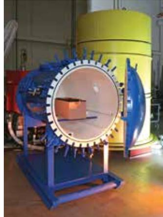
SwRI battery test facilities include altitude chambers.
