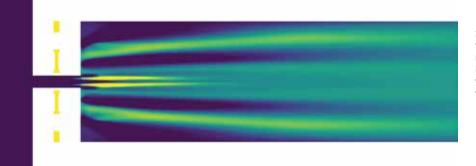
SwRI is exploring the use of "green" hydrogen fuel for gas turbines used to generate power. The designs include a nozzle that rapidly mixes and injects air (dark blue in the image) and fuel (yellow in the image) into the combustor to prevent flashback, a common hazard in hydrogenfueled power generation applications.
