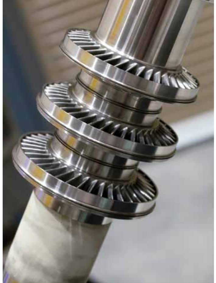
SwRI designed and manufactured this unique sCO<sub>2</sub> turbine for installation into the STEP demonstration pilot plant. Testing will begin later this year.
