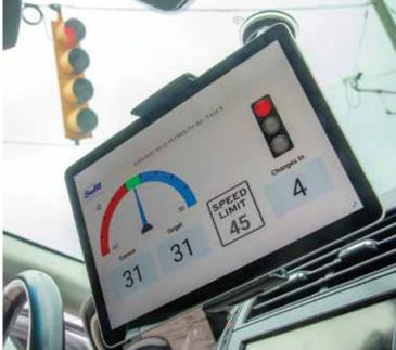
SwRI developed an eco-mobility app that uses roadway connectivity data to advise drivers to speed up or slow down to avoid red lights. Significantly more energy is required to accelerate vehicles, particularly heavy-duty trucks, after making a full stop at lights.
