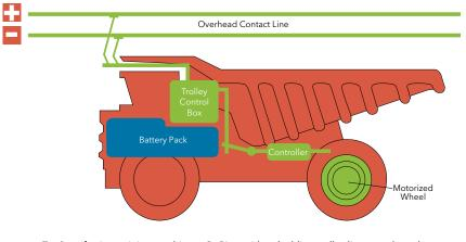
To electrify giant mining machinery, SwRI considered adding trolley lines to selected segments of the delivery route to charge onboard battery packs while trucks are in service, allowing the haulers to operate 24/7.
