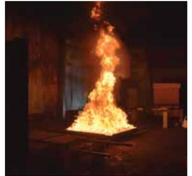
Fire specialists expose fully charged electric vehicle batteries to gasoline pool fires.
