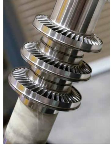
SwRI designed and manufactured this unique sCO2 turbine for installation into the STEP demonstration pilot plant. Testing will begin later this year.
