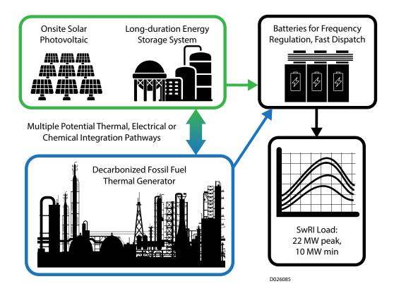
**DETAIL** Frequency regulation balances electricity supply and demand at all times, particularly over time frames from seconds to minutes. Fast dispatch sources of electrical power can be rapidly accessed or turned on to meet demand.
