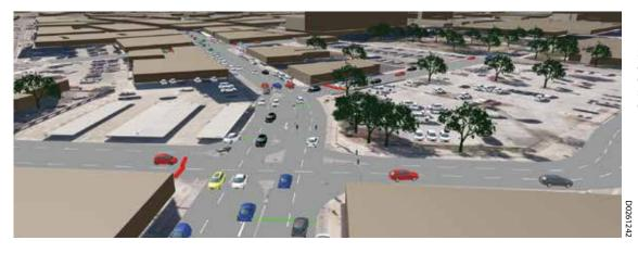
SwRl's connected and automated vehicle chassis dynamometer uses traffic simulation software to evaluate eco-mobility tools.
