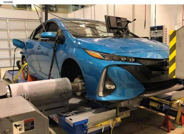
Located in SwRI's Ann Arbor, Michigan facility, SwRI's connected and automated vehicle chassis dynamometer runs a vehicle in response to traffic data. A data acquisition system collects relevant operating data to determine the efficiency improvements.
