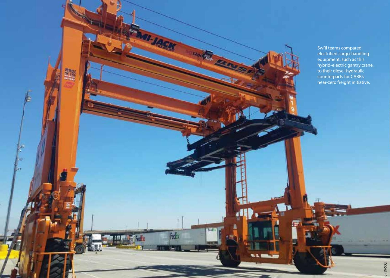
SwRI teams compared electrified cargo-handling equipment, such as this hybrid-electric gantry crane, to their diesel-hydraulic counterparts for CARB's near-zero freight initiative.
