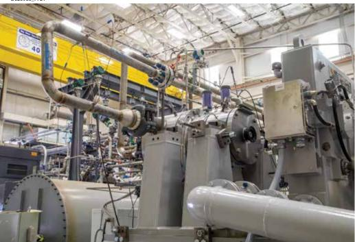
SwRI engineers developed a 3 MWe sCO<sub>2</sub> turbine for geothermal applications and integrated the machinery into a production rig.
