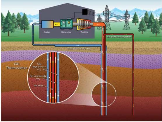
This schematic of a geothermal thermosiphon illustrates its  $CO_2$  injection leg,  $CO_2$  production leg, surface equipment and brine reinjection leg configuration.
