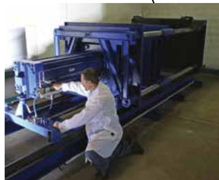
SwRI developed equipment to crush test whole battery packs (pictured) as well as fixtures to crush test individual cells.
