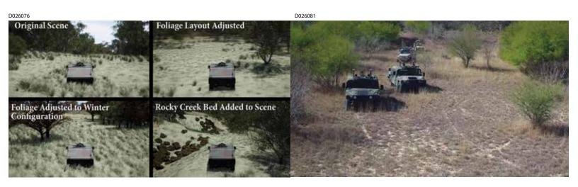
SwRI's Simulation Scene Adjustment Tool evaluates automated vehicles in 3D simulations of off-road environments. The image shows 3D scenes featuring different ground cover, simulating grass, foliage or rocks to virtually test military automated ground vehicles (AGVs).
