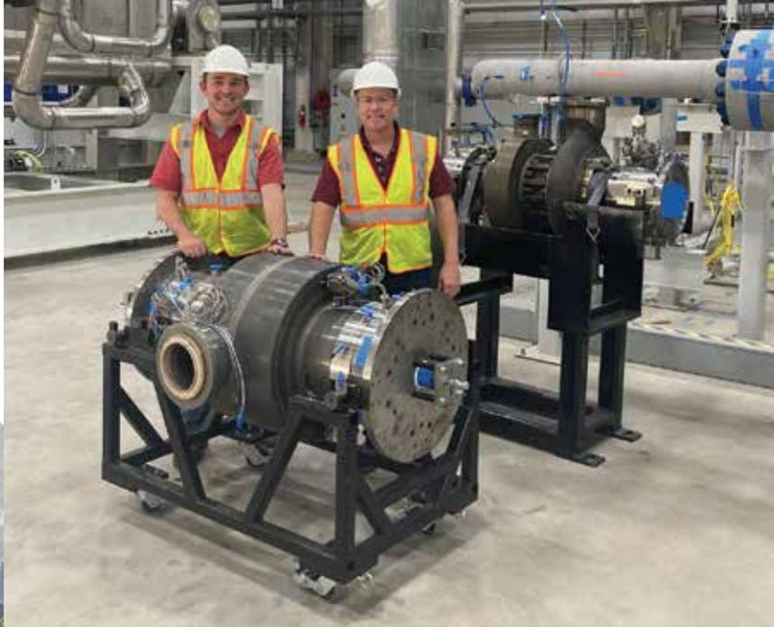
SwRI's John Klaerner, left, lead turbine engineer, and Dr. Jeff Moore, right, principal investigator of the STEP Demo project, are pictured with the recently assembled sCO<sub>2</sub> turbine for the 10 MWe demonstration plant under construction at SwRI.
