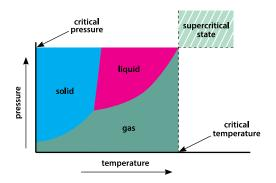
The supercritical temperature of a substance is the temperature where gases cannot become liquid, regardless of the applied pressure. (See related story on p. 14) D026139
