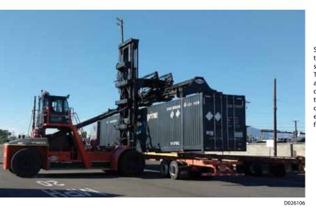
SwRI used dataloggers to monitor this electric side pick cargo handler. The project collected almost a million rows of data each day for analysis to help a commercial client optimize its electrification plans for freight equipment.
