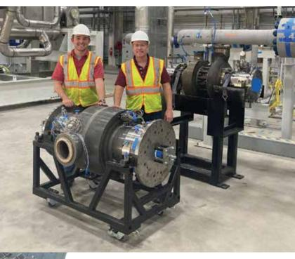
SwRI's John Klaerner, left, lead turbine engineer, and Dr. Jeff Moore, right, principal investigator of the STEP Demo project, are pictured with the recently assembled  $sCO_2$  turbine for the10 MWe demonstration plant under construction at SwRI.
