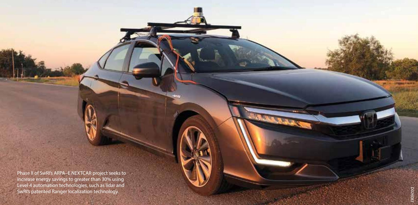
Phase II of SwRI's ARPA-E NEXTCAR project seeks to increase energy savings to greater than 30% using Level 4 automation technologies, such as lidar and SwRI's patented Ranger localization technology.
