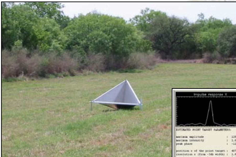
Corner reflectors, such as this one developed at SwRI, can be installed in areas that do not contain sufficient natural radar measurement points (for example, in highly vegetated, snow-covered and low infrastructure areas). These trihedral or dihedral structures have panel sizes of approximately 1 x 1 m (for C-band satellite data).
