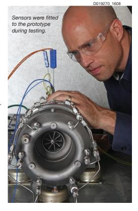
tuning to meet the machine requirements. *In-situ* rotor system balancing resulted in very low vibration levels, and the compressor met aerodynamic performance predictions.
