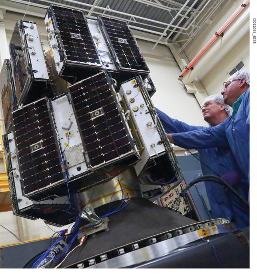
SwRI engineers prepare NASA's eight Cyclone Global Navigation Satellite System (CYGNSS) microsatellites, mounted on the deployment module, for vibration testing.
