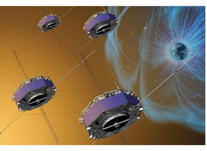
Launched March 12, 2015, the four identical MMS spacecraft skim the sunward boundary of Earth's magnetosphere in a close tetrahedral formation. Each spacecraft carries a payload of 25 instruments to measure with unprecedented resolution the plasma, energetic particles, and electric and magnetic fields near and in magnetic reconnection sites.
