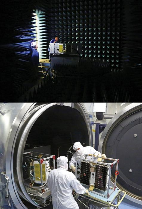
Top: SwRI is designing, fabricating, and integrating the CYGNSS constellation of eight microsatellites.
