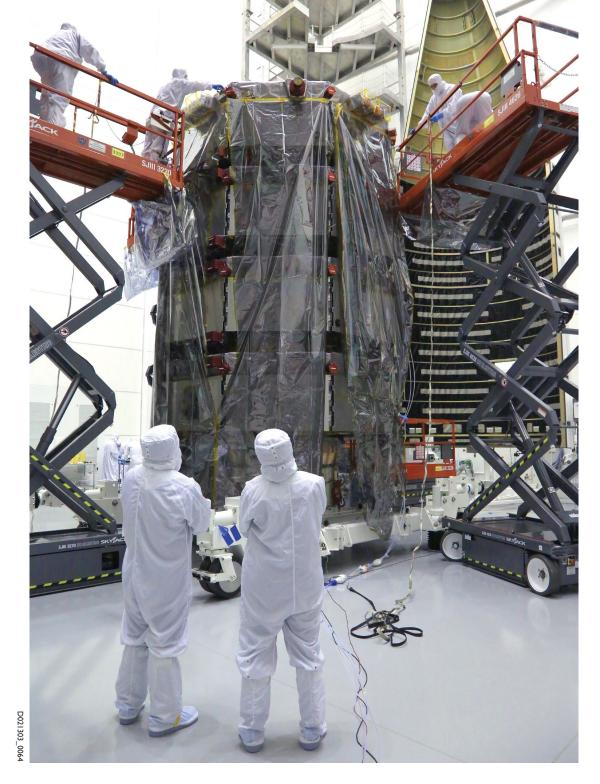
Each of the four MMS observatories is octagonal in shape, approximately 11 feet across by 4 feet high.When stacked together inside the Atlas V launch vehicle, the observatories are more than 16 feet tall.
