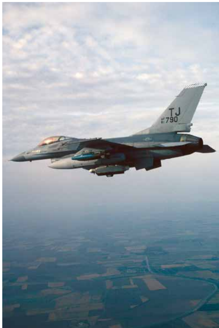
This F-16 aircraft is outfitted with an ALQ-131 electronic attack pod to provide electronic warfare protection. Institute staff members have comprehensive background and expertise in active and passive electronic warfare systems.
