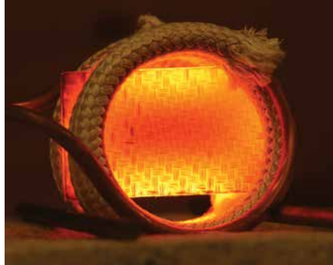
As part of its hypersonics research, SwRI is conducting high-temperature materials testing of carbon-carbon composites, shown glowing at 2,000° F.
