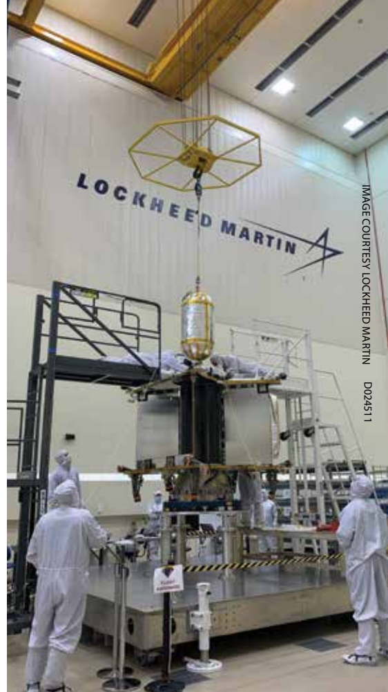
Engineers install Lucy's oxidizer tank into the spacecraft structure in the high bay at Lockheed Martin.
