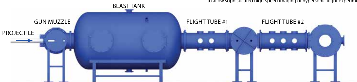
SwRI's light-gas gun flight range includes multiple portals in the flight tubes to allow sophisticated high-speed imaging of hypersonic flight experiments.
