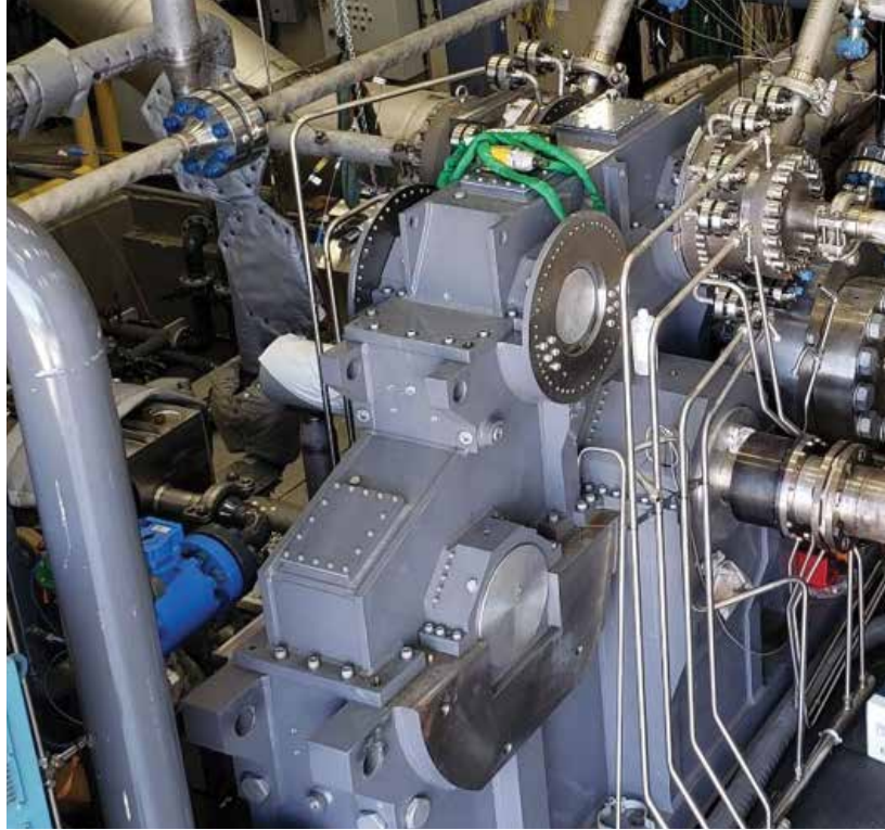
Engineers are testing an integrally geared compressor-expander prototype for its performance and durability.
