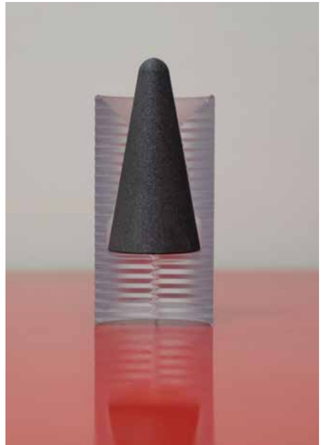
For light-gas gun testing, SwRI encases spherically blunted conical test projectiles in a sabot, a structural device used to keep smaller projectiles in the center of the barrel when fired. The sabot separates from the projectile and is stripped away when it hits an impact plate.
