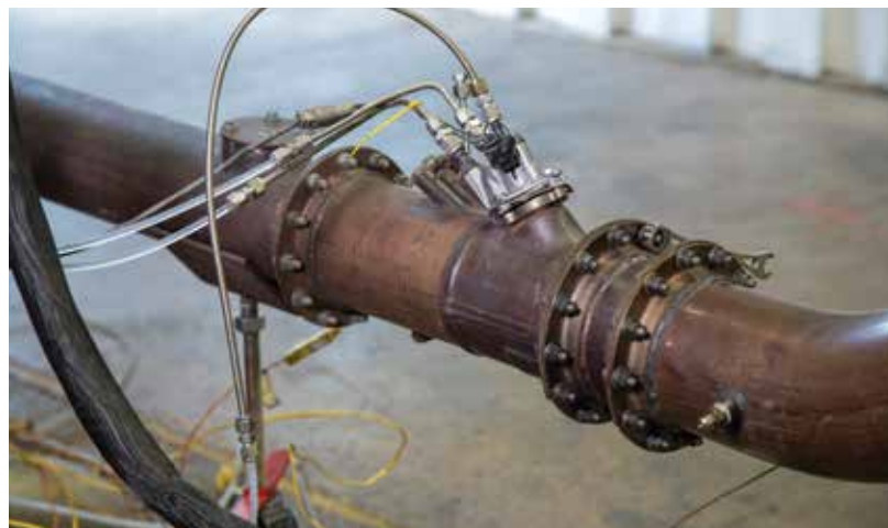
SwRI's Cat-DEF™ technology was recognized for reducing nitrous oxide (NOx) and carbon dioxide emissions by minimizing deposit formation in diesel engine exhaust systems.
