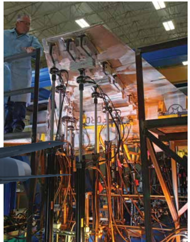
Since the 1960s, the Air Force has structurally modified the fuselage of its advanced flight trainer, the T-38 aircraft (left), to extend its structural life. SwRI conducted a full-scale structural fatigue test, destructive teardown and economic life evaluation to help assess remaining life and identify potential fatigue-critical locations.
