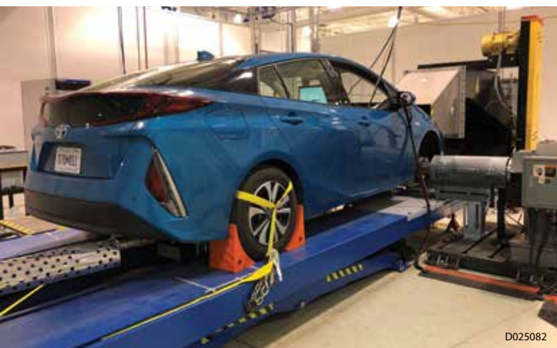
SwRI developed a connected and automated vehicle (CAV) chassis dynamometer that interfaces with traffic simulation software to provide a controllable, repeatable environment for testing tools.
