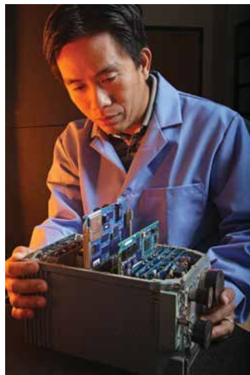
The SwRI-developed Improved Electronic Processing Unit combines engine turbine monitoring and aircraft structural integrity systems into a single, consolidated line-replaceable unit for the entire A-10C fleet.
