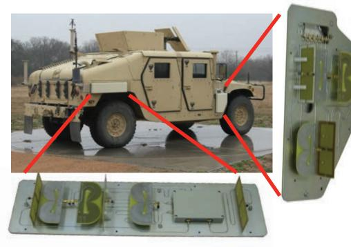
The sub-arrays—with one facing front, rear and two broadside—work together to provide 360-degree coverage. Two different antenna element types are used: balanced-shielded loop antenna elements to cover VHF frequencies and tapered-slot antenna (TSA) elements for UHF. Each sub-array design was 30 inches long by 7.5 inches tall by 3.5 inches deep for this platform.
