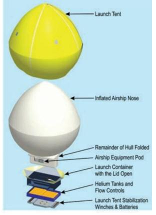
The TALS package comprises the airship, protected within a launch tent, along with all equipment required to launch it.
