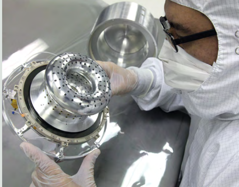
SwRI designed Strofi, a basketball-sized instrument weighing just over 7 pounds, to measure particles in Mercury's sparse exosphere.
