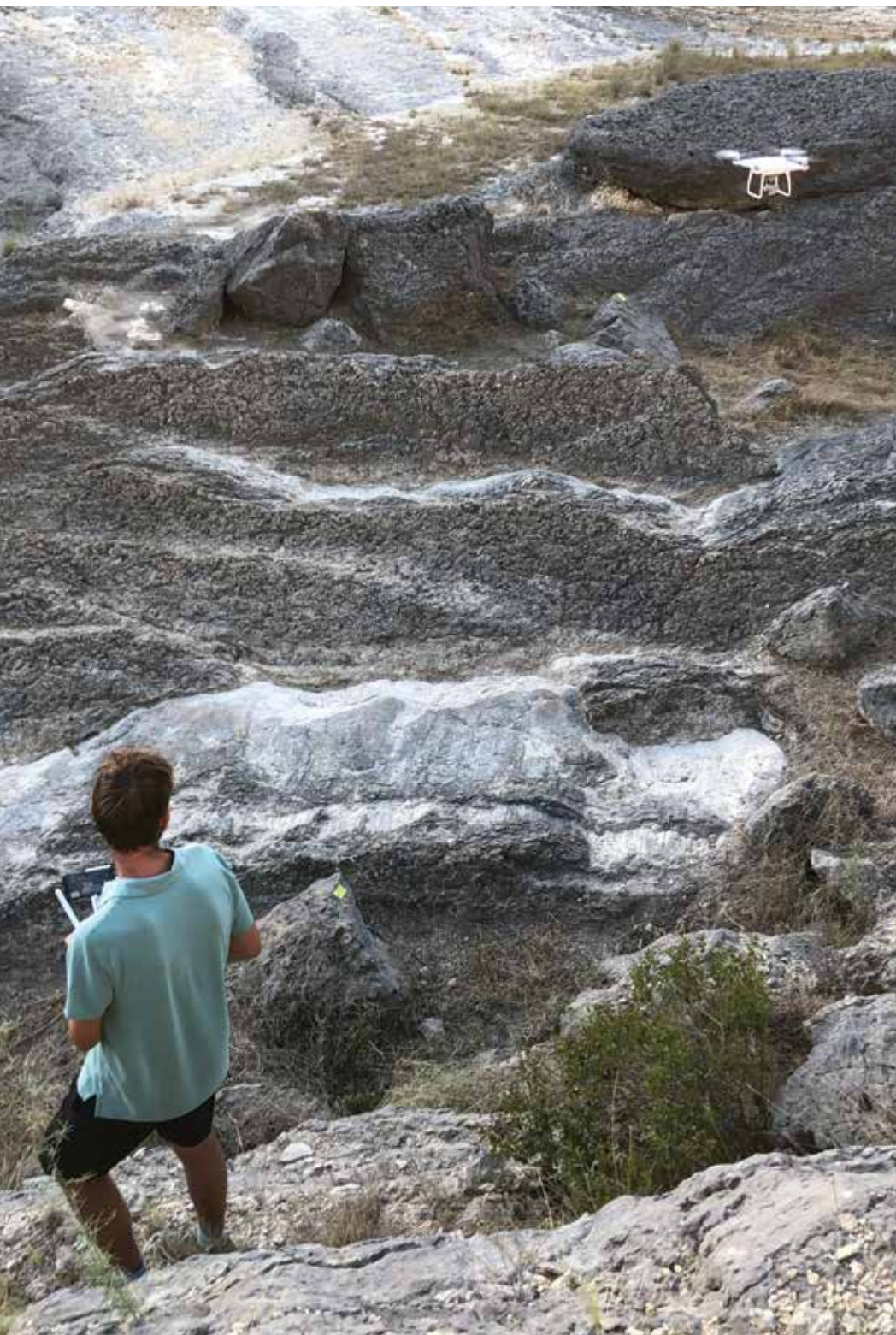
SwRI's Dr. Adam Cawood collects UAV imagery of surface rock exposures with precise GPS data to build high-resolution, accurate "digital outcrops" for geological data extraction.
