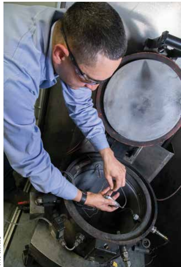
Staff Technician Mario Guillen installs a lithium-ion battery cell in a calorimeter to evaluate the thermal stability limit for battery cells and calculate heat release during failure.
