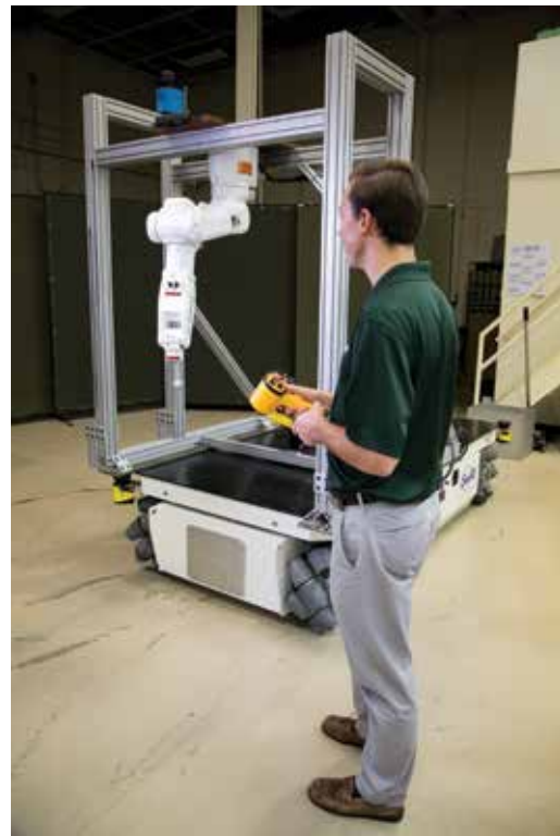
Engineers developed a small-scale mobile manipulator system to demonstrate using an off-the-shelf industrial manipulator, mobile platform and metrology system. The system was adapted for picking up and sorting items in a warehouse application.
