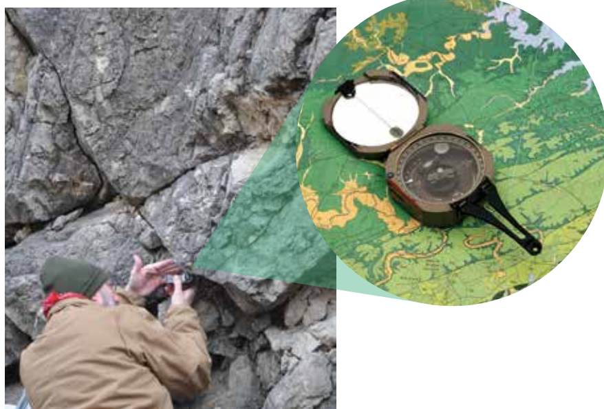
SwRI geologist Dr. Kevin Smart uses a compass clinometer to measure fault orientations by hand.
