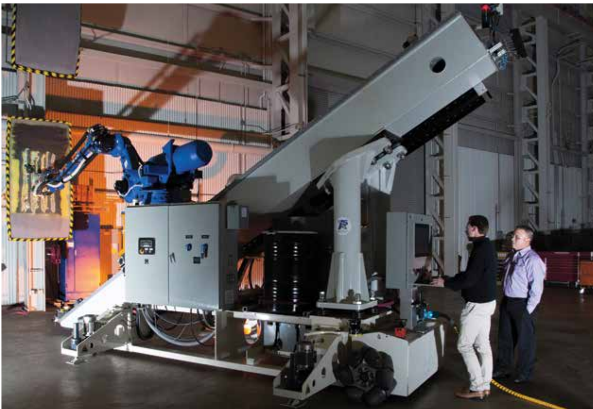
SwRI demonstrates the A5 Robotic System, a mobile platform designed for adaptability and flexibility for a range of aircraft manufacturing and maintenance activities, including surface processing.
