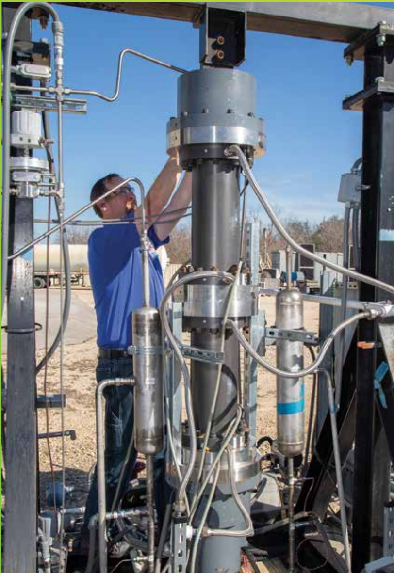
Senior Research Engineer Nathan Poerner performs maintenance on the hermetically sealed LMRC that SwRI designed for hydrogen compression.
