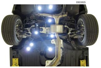
This research vehicle is equipped with SwRI's Ranger localization technology for automated vehicles. Using a ground-facing camera, illumination, and algorithms, Ranger allows for precise automated driving, accurate to within 2 centimeters.
