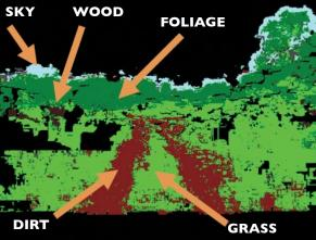
SwRI's unmanned vehicles use a low-cost sensor suite and sophisticated software to identify pedestrians and distinguish between terrains, such as dirt, roadway, grass, and sky.
