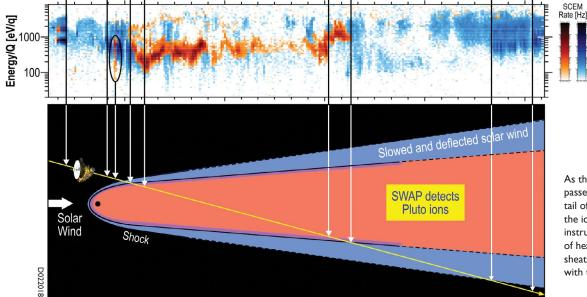
As the New Horizons spacecraft passed beyond Pluto, it traversed a tail of heavy ions emanating from the icy planet. The SWAP instrument measured a population of heavy Plutogenic ions (in red) sheathed in lighter ions associated with the solar wind (in blue).
