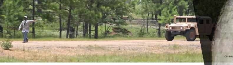
SwRI developed gesture recognition capabilities for unmanned vehicles used in military, highway work convoy, and other applications. Image-processing algorithms identify and distinguish different arm gestures from a designated pedestrian to give commands that allow more natural, efficient interaction with an automated vehicle.
