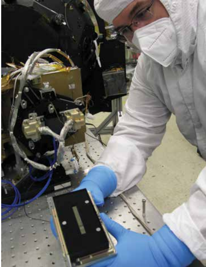
An SwRI team including Lead Scientist Dr. Todd Veach built the MVIC camera, the only visible light multicolor imager in Lucy's payload.
