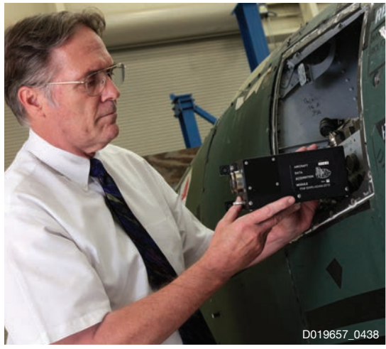
SwRI-designed-and-built recorders are mounted in aircraft to gather structural load data.
