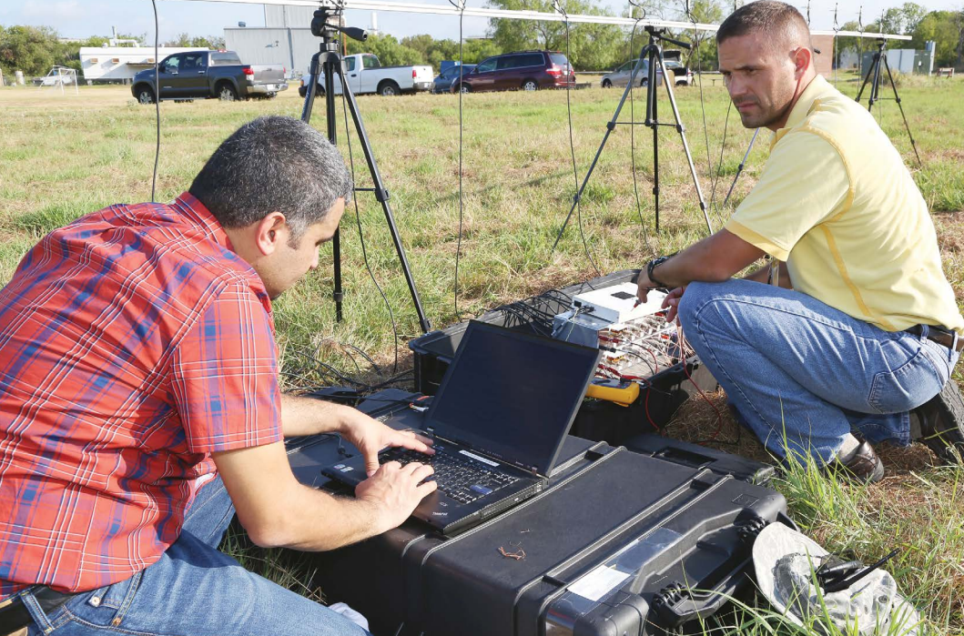
Dayeh and Engineer James J. Ramaekers calibrate an “acoustic camera,” an array of 15 microphones set 1 meter apart and mounted on tripods 1.2 meters above the ground.
