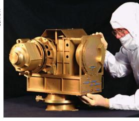
SwRl operated two of Cassini's 12 science instruments, as part of the fields, particles, and waves experiment package. The Cassini Plasma Spectrometer (CAPS), above, and the Ion and Neutral Mass Spectrometer (INMS), below, both studied plasma in the Saturn system. While they didn't produce actual "pictures," the information they collected is critical to scientists' understanding of the Saturn system, including its moons and rings.
