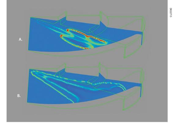
SwRI frequently uses computational fluid dynamics to understand the dual-fuel combustion process. Frame A shows the initial diesel ignition, while Frame B shows later diffusion burning of the diesel plume inside, with natural gas flame front on the outer edges.
