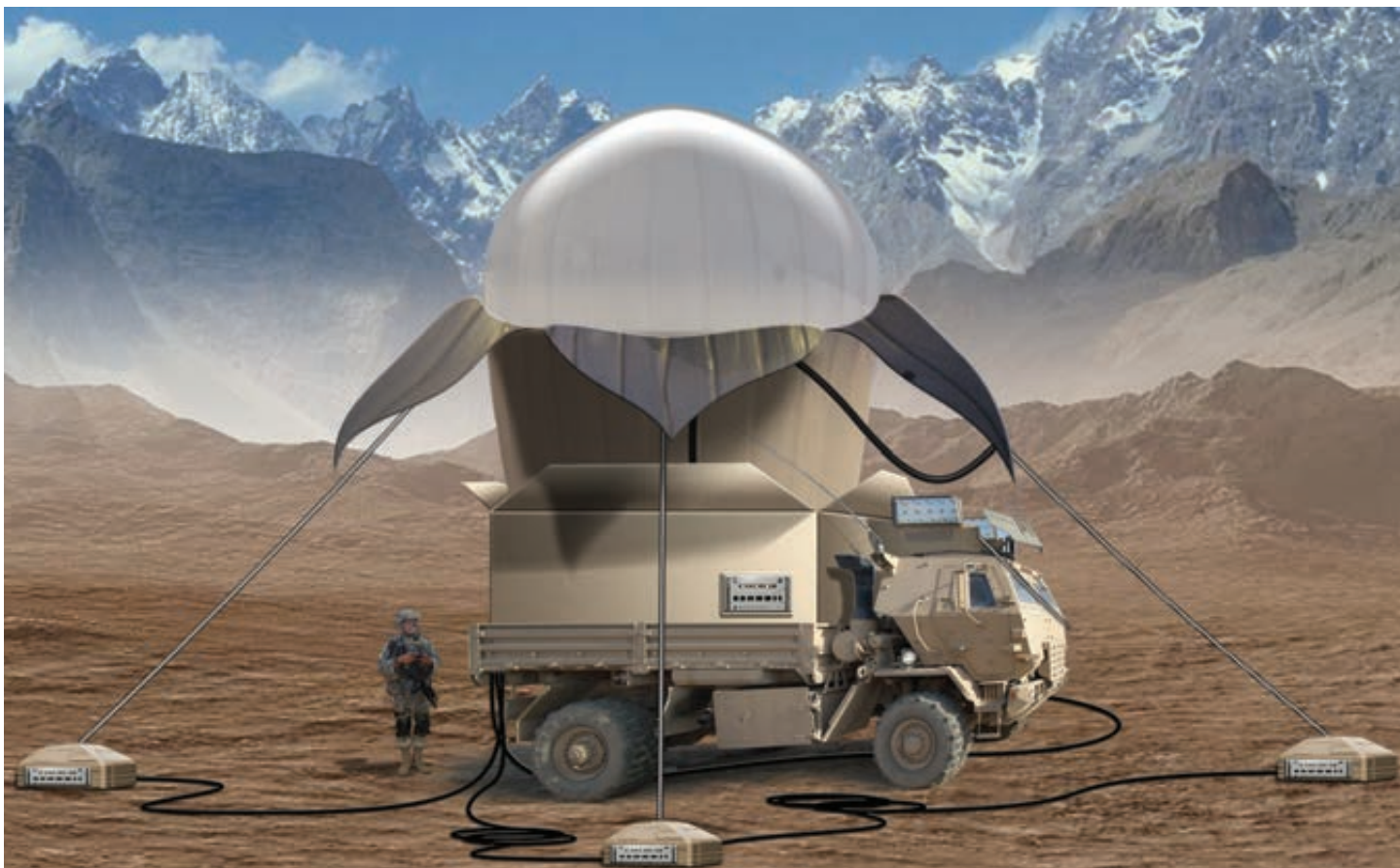
In this artist's rendition, a truck-transported container serves as the inflation and launch platform for a TALS application in an austere environment.
