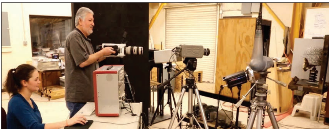
The test setup includes ballistic light screens to measure impact velocity, a digital chronograph to measure time, a universal gun mount system, high-speed video cameras and flash X-ray imaging systems, among other instrumentation.
